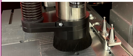
Dust shoe for Ø 65 mm spindle
