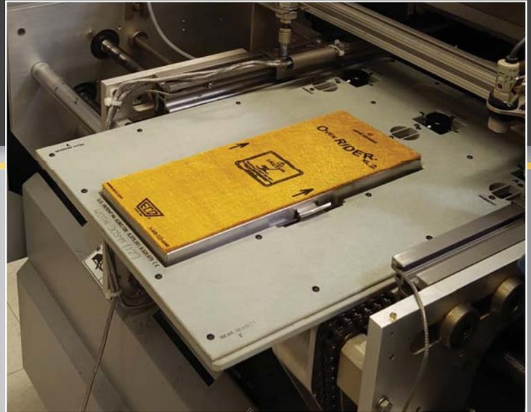
The patented OvenRIDER® NL 2+ travels through your oven with a M.O.L.E.® inside collecting data for analysis and SPC charting. A combination of thermal and process sensors measure oven performance, delivering consistent data that can be used to identify modest trends which may be developing, or serious conditions that have already arrived. Simple PCB profiling cannot detect all the subtleties which can have a profound effect on PCB production quality.
