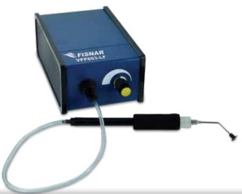
For delicate handling of small parts and components, including miniature, surface mount and chip scale packages. Designed to capture the part and to place the component gently in position. Closing a small hole in the hand-piece with your finger creates the vacuum. To release, uncover the hole by removing your finger.
