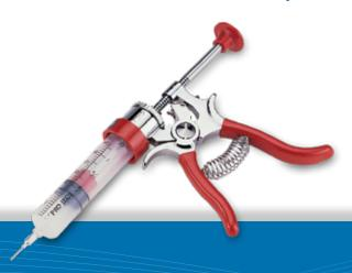
The AD93 volumetrically dispenses epoxies, silicones, glues and pastes. Available in two capacities, 35cc and 80cc syringe, with hot stamped sidewall indicators for dosage levels in cc and ounces. Shot sizes can be selected in increments of 1cc to 5cc. Material delivery is via luer lock tips.
