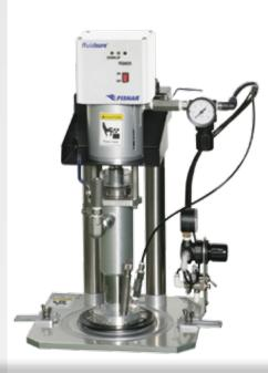
The EP1301N is designed for a 1kg (1qt) can of medium to high viscosity fluid. The EP1303N is configured for a 3kg (1 gallon) can of similar viscosity. Both systems are rated at 15:1 and provide a maximum of 996psi regulated material pressure.
