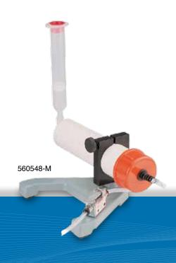
The model 560548-M loads a barrel directly from a 1/10 gallon caulking tube. The barrel loader is connected to an air regulator and set to a pressure suitable for the material but less than 65psi (4.48 bar). A switch on the side of the stand activates the airflow and is switched off when the material reaches the desired level. The barrel attachment assembly is threaded to accept luer lock barrels.
