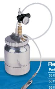
The needle valve pen simplifies the application of a low to medium viscosity fluid, which is not affected by contact with metal parts. Material is fed into the pen from a cartridge or reservoir. The finger control shut off instantly opens and closes the material flow. The pen is suitable for microdots, beading and potting operations.
