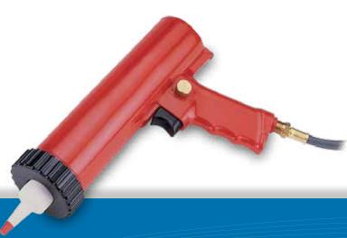
Dispense caulk and sealant materials. Connect the 580112C to a regulated air supply to dispense directly from the caulking tube. Most materials will dispense satisfactorily from 12 to 30 psi (0.80 - 2.0 bar). Do not exceed 60 psi (4 bar).
