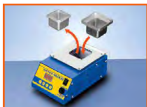
Change the pot and tighten the screws.
