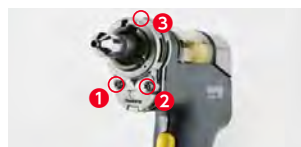
By removing 3 screws
