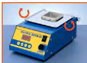
Loosen the screw on both sides.
