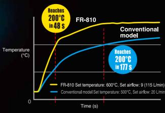
\*Examination of time taken for connector sections soldered onto a ceramic board to be heated to 200 °C with maximum temperature and
