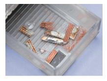
After cutting, the wick debris (or sliver of wick) is collected in the wick collector, preventing them from scattering onto the workbench and eliminating contamination concerns.
