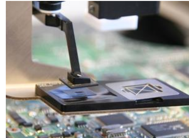
BGA on Placement Nozzle after Flux Dipping.
