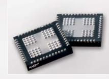
QFN interconnects prebumped with solder paste.
