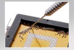
Easy distribution of solder spheres (solder balls) on a universal mask. Excess spheres are simply poured back into container.
