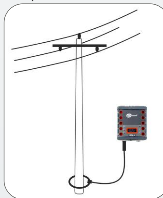
Device working with single clamp.
