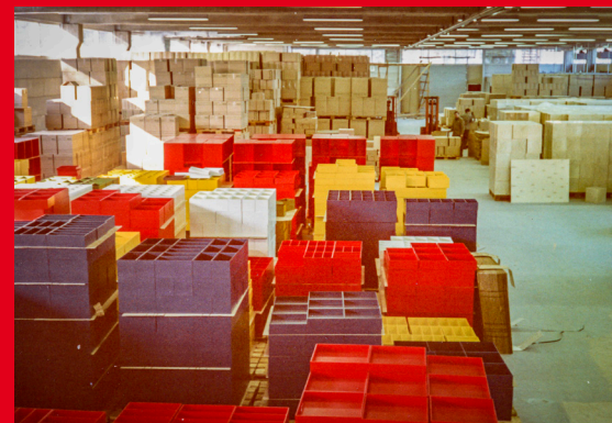
All newly made Palaset modules were light brown in colour. A coat of paint was needed to give them their distinctly bright and cheerful look.
